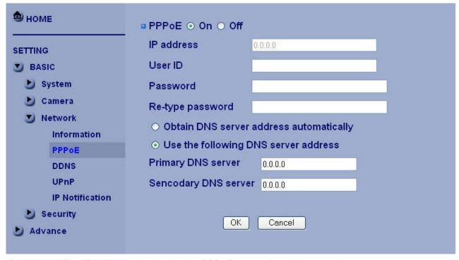
IP address: The IP address obtained at the PPPoE connecting with network.
